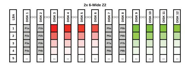
As in the Z3 diagram, each data stripe gets its own pair of unique parity sectors. The first data block is written to the first vdev and the second data block is written to the second vdev. A third data block would again be written to the first vdev, and so on.
