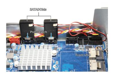
Both SATADOMs are powered from one cable attached to the *Front\_USB* header on the motherboard. Use thumb and index finger to grip the USB power connector and gently pull upward to disconnect.
