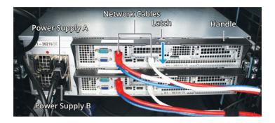
Grip the handle and pull to remove the node completely. Gently lift the node and place it on an antistatic surface.
