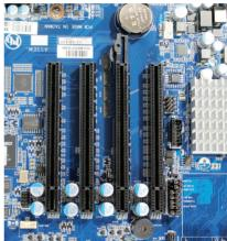
Align the four edge connectors with the PCle slots on the motherboard. Press down evenly on the PCle Bus Riser until the edge connectors click into place and are firmly seated.
