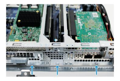
Place thumbs on the top corners of the Front Plate and push upward to partially release the PCIe Bus Riser from the motherboard.
