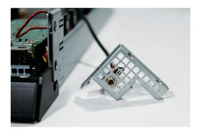
Remove the two screws to detach the left slot cover retainer. Set retainer and screws aside for use later.
