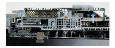
Locate the PCIe Bus Riser release latch. Press on the release latch while lifting the PCIe Bus Riser to remove it completely.
