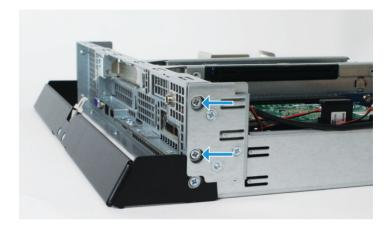
Place the slot cover retainer next to the node with the wires still attached. Save the screws.
