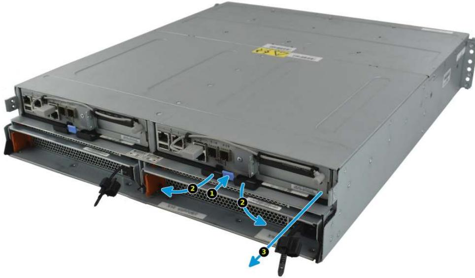
Swing the levers open on the replacement controller, then gently slide the controller into the chassis until it stops. Gently swing the levers closed to lock it in place.
