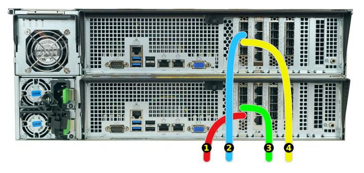
Connect SAS cables to the ES12 T slots. These are the typical SAS connections for one or two ES12 expansion shelves connecting to a High Availability (HA) TrueNAS<sup>®</sup> system with two storage controllers. When a TrueNAS<sup>®</sup> unit with only a single storage controller is used, only cables #1 and #3 are connected.
