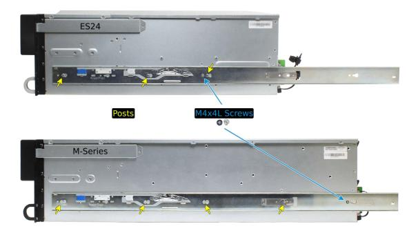
Align the rail hole with the screw hole and secure the rail with one M4x4L screw from the rail kit. Repeat this process to mount and secure the second cabinet rail on the other side.
