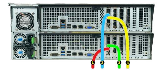
The SAS cables from the TrueNAS® system connect to these ports on the ES24:
