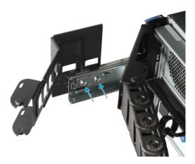
Locate the end of the flex housing with exposed holes. Unclip and open the two tabs closest to the end, allowing the flex housing to expand enough to fit over the bracket pins. Press the flex housing firmly into the bracket until the holes seat on the pins.
