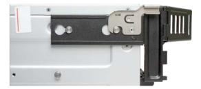
Locate the end of the flex housing with exposed pins. Unclip and open the two tabs closest to the end, allowing the flex housing to compress enough to fit into the bracket holes. Press the flex housing firmly into the bracket until the pins seat in the holes.
