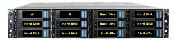
To load an individual drive tray into a bay, press the blue button to open the latch. Carefully slide the tray into a drive bay until the left side of the latch touches the metal front edge of the chassis, then gently swing the latch closed until it clicks into place.
