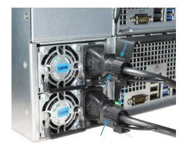
After both power cords have been connected to the M-Series, they can be plugged into power outlets. The system is configured to automatically power on when connected to a power outlet. This design ensures that the M-Series comes back on when power is restored after a power failure.
