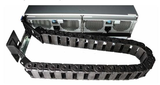
Power and data cables are routed through the flex housing. The tabs can be opened or removed to allow access or space for cable ends. Leave some slack in the cables at both ends to allow for movement of the arm and chassis.
