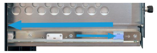
To secure the drive bay and prevent it from accidentally opening, tighten the captive thumbscrews on the front of the system. You can also use the included key to lock the drive drawer and prevent unauthorized access.
