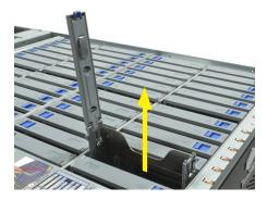
The R50 is certified to use WD Helium drives only. Align a hard drive with the connectors facing downwards into the system, then slide the drive into the slot. Squeeze the plastic release tabs on each side of the tray, then push the tray downwards to install the hard drive into the system. Close the slot cover and make sure it locks.
