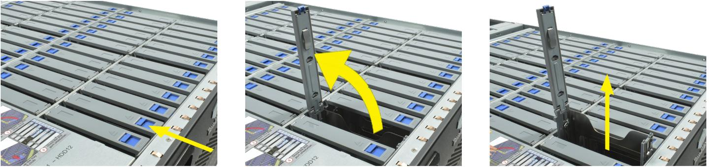
The R50 is certified to use WD Helium drives only. Align a hard drive with the connectors facing downwards into the system, then slide the drive into the slot. Squeeze the plastic release tabs on each side of the tray, then push the tray downwards to install the hard drive into the system. Close the slot cover and make sure it locks.
