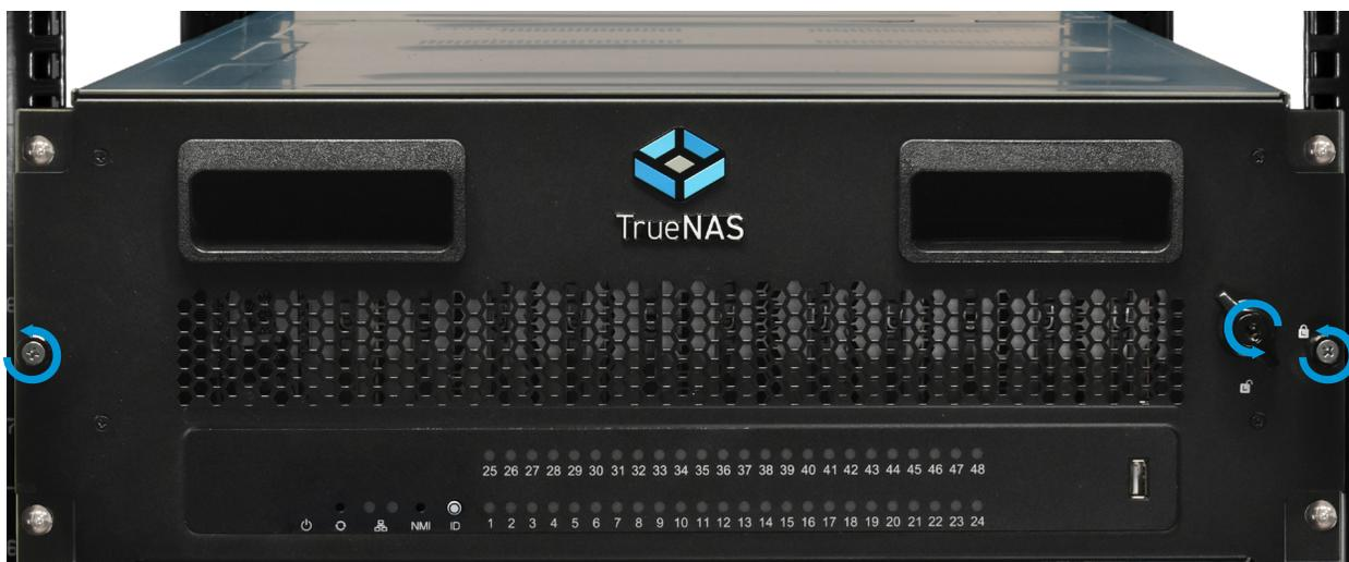
Pull the blue release catches on each rail toward you, then pull the drawer out of the system.
