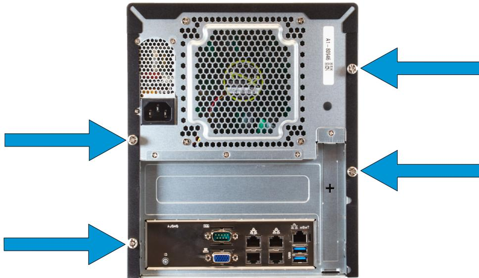
Slide a side panel off the chassis by grasping the side and pulling the panel away from the front of the system. When the side panel can no longer move away from the chassis frame, gently pull the panel away from the system.
