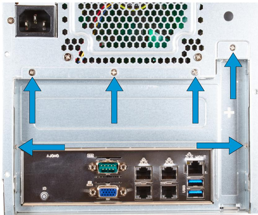
Very carefully pull the tray out of the back of the system. Continuously check that no wires are being pulled or caught on other components inside the system.
