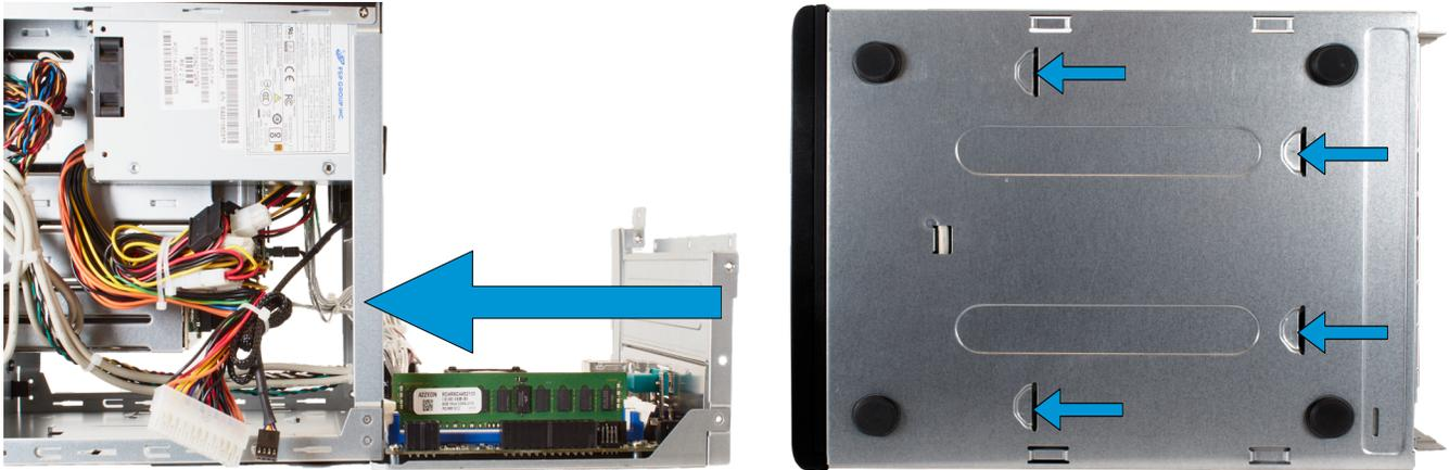
Re-attach the screws on the back of the chassis to secure the motherboard tray in place.
