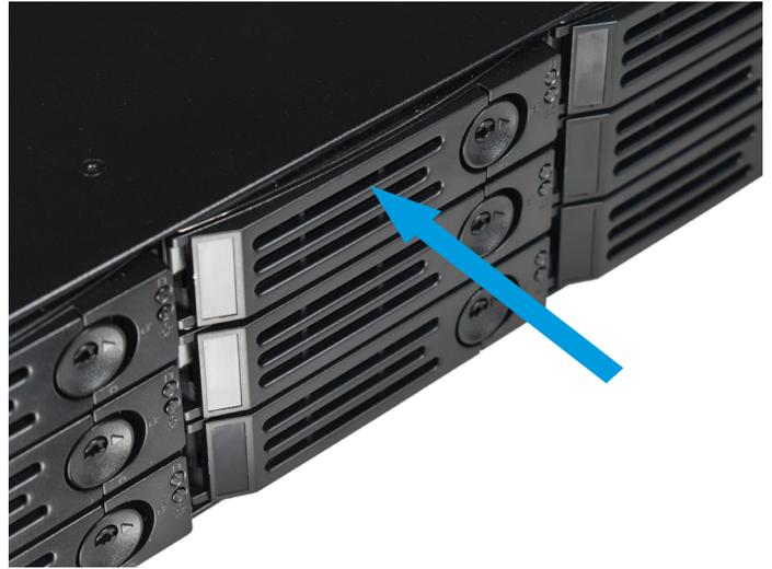
For extra security, you can lock the drive tray into the system. The tray button is unlocked when the inner slot is horizontal and locked when the slot is vertical. To lock a tray, insert a flat-head screwdriver into the center button slot and gently turn it ninety degrees clockwise until the slot is vertical.
