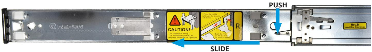
Align the chassis rail on the side of the system designated by the stickers and ensure they are right-side-up. Place the rail slots over the chassis tabs, then slide the rail toward the front of the system until it clicks into place. Secure the rail to the system using one of the low profile #6 rail screws. Repeat this process for the other rail.
