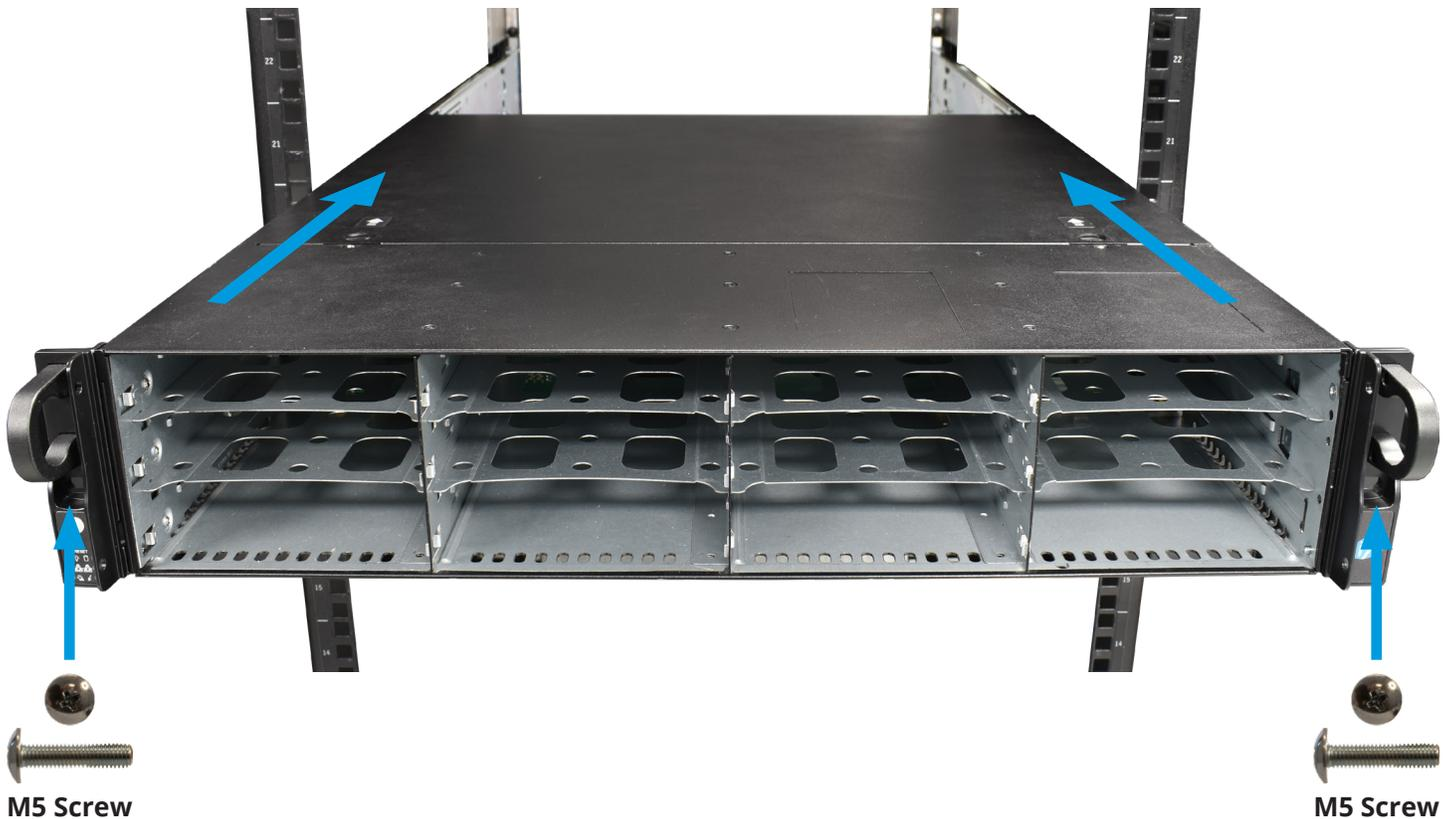
Insert a long M5 screw through the holes on each ear to secure the Mini R to the rack.
