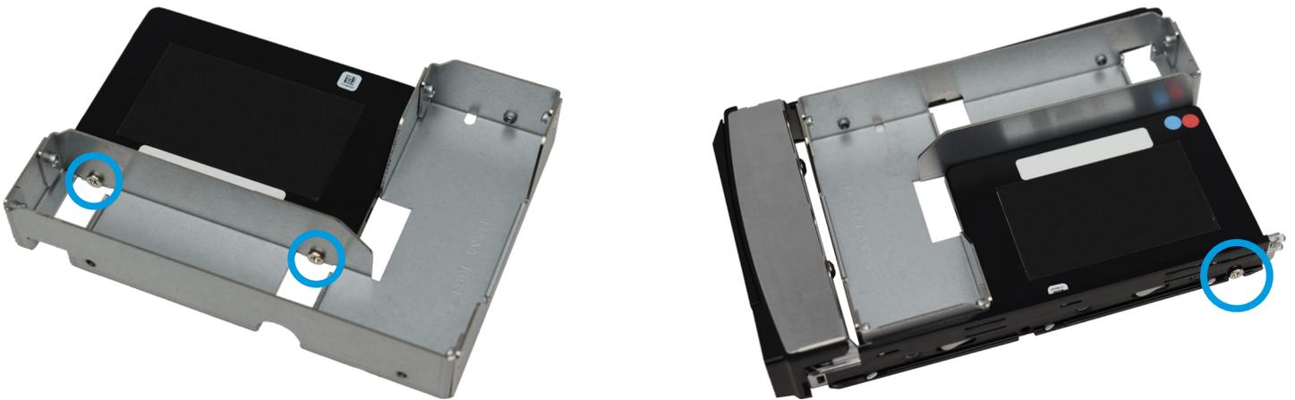
Use three HDD screws to attach the adapter and SSD to the drive tray.
