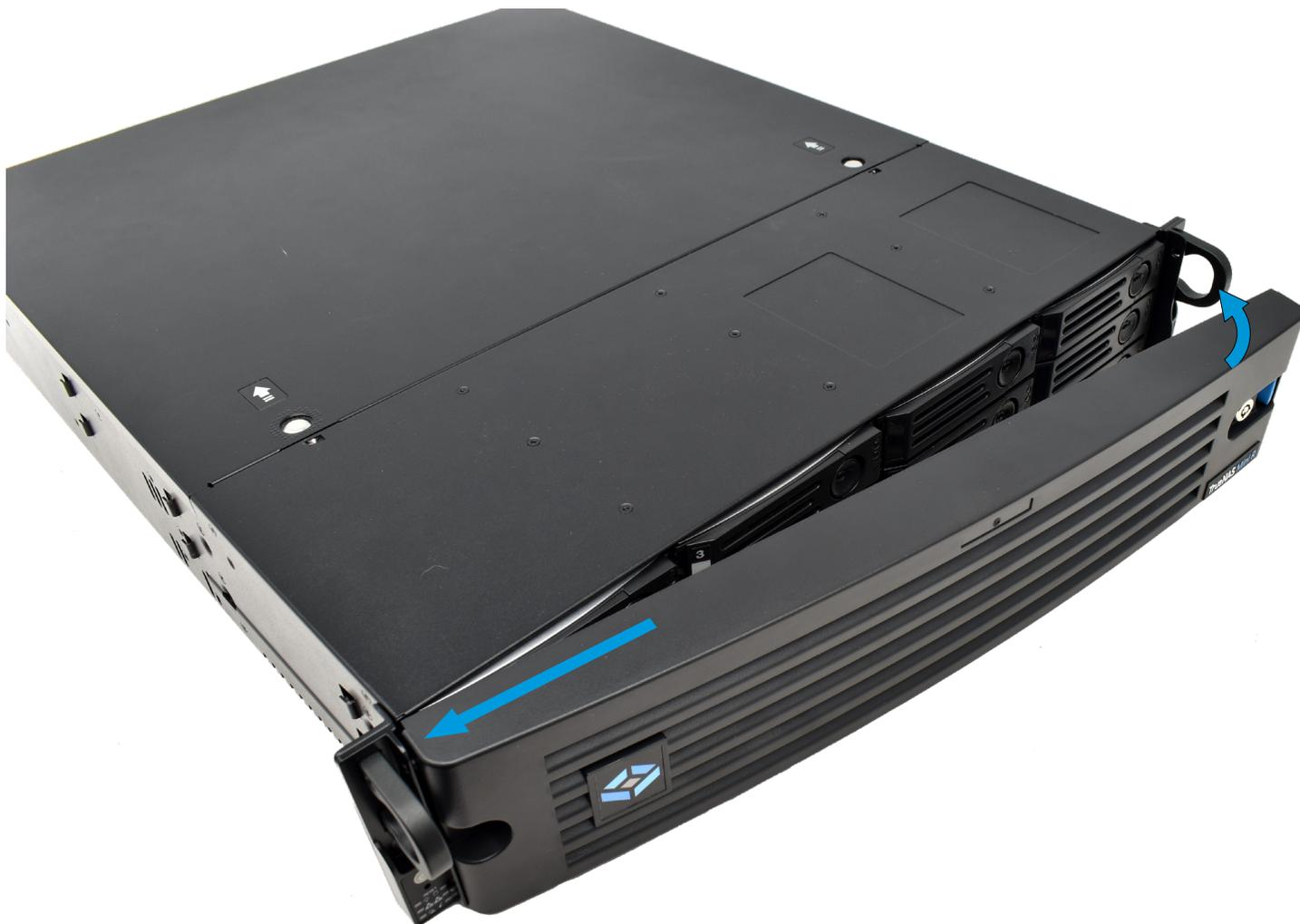
You can lock the bezel for added security. To do so, insert a key in the lock and turn it ninety degrees clockwise.
