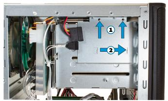
Mount an SSD in the tray with four small screws, one at each corner. Make sure the SSD power and SATA connectors are pointed towards the back of the tray so the cables can be properly attached.
