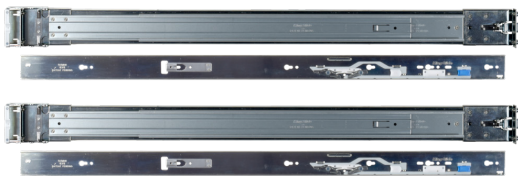
Set of rackmount rails. The rails have a specific front end, identified by a label visible on the left above. The front ends of the rails must be installed facing the front of the rack.
