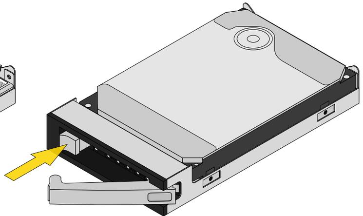
Align the drive assembly with an empty slot on the system and push it in until the locking arm begins to swing closed. Gently close the arm to fully seat the drive tray and lock it into the system.
