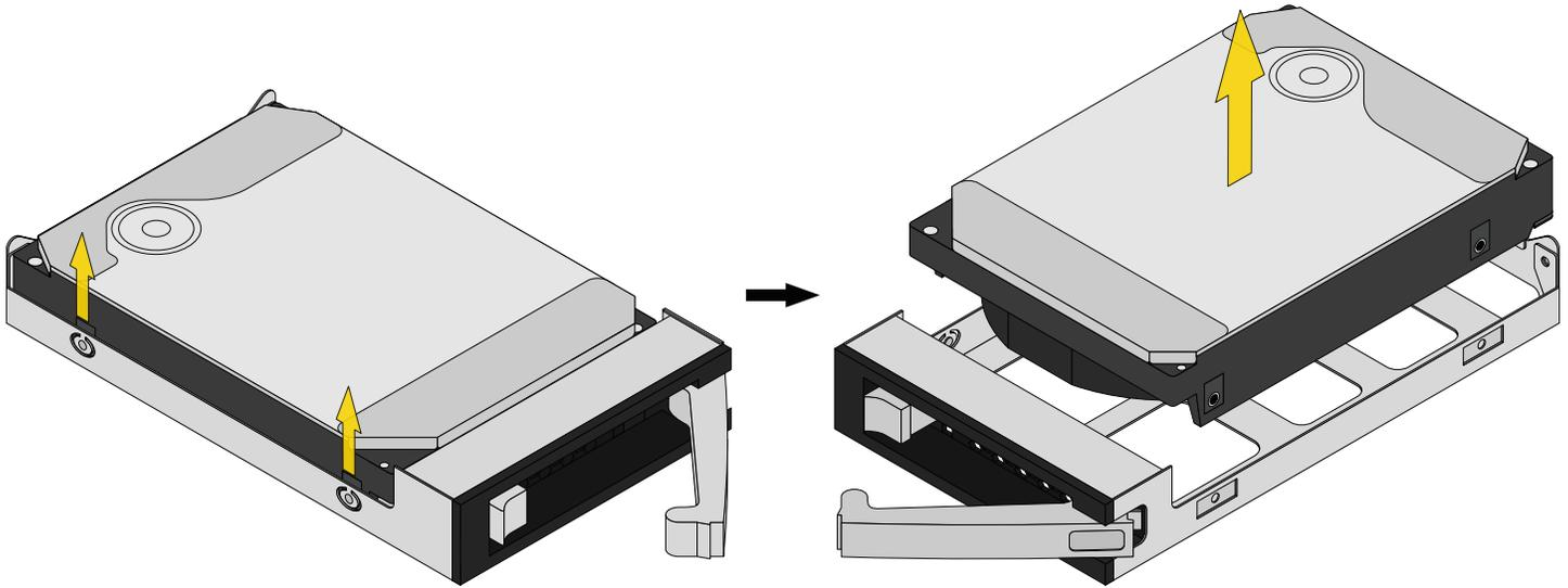
To install a drive in a tray, ensure the drive connectors point out the back of the tray and push the drive side screw holes into the fixed retention pegs on one side of the tray.
