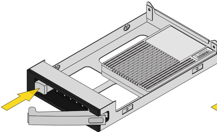
Drive Assembly with HDD
