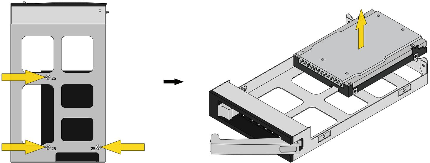
To install an SSD in a tray, ensure the drive connectors point out the back of the tray, then lower the drive into the tray. Install three 2.5" SSD screws to secure the drive to the tray.
