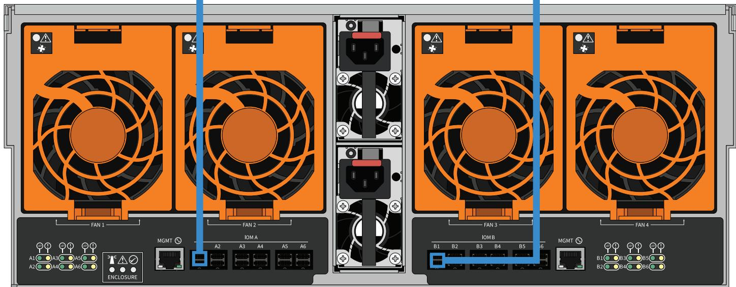
M50/M60 with three ES60 Expansion Shelves. The M50 can support up to 8 total Expansion Shelves with the use of additional SAS cards. The M60 can support up to 12 total Expansion Shelves with the use of additional SAS cards.
