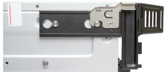
Locate the end of the flex housing with exposed pins. Unclip and open the two tabs closest to the end so the flex housing can compress enough to fit into the bracket holes. Press the flex housing firmly into the bracket until the pins seat in the holes.
