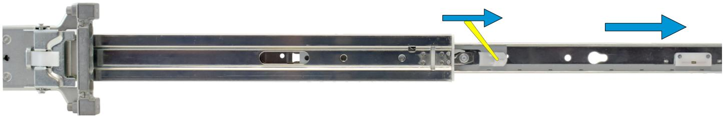
The chassis rails mount on each side of the system. Align the chassis rail keyholes with the posts on the side of the chassis. Slide the rail towards the system rear until the metal tab clicks and locks the rail in place. Secure the rail to the chassis using the low-profile M4 screws. Repeat this process on the other side.
