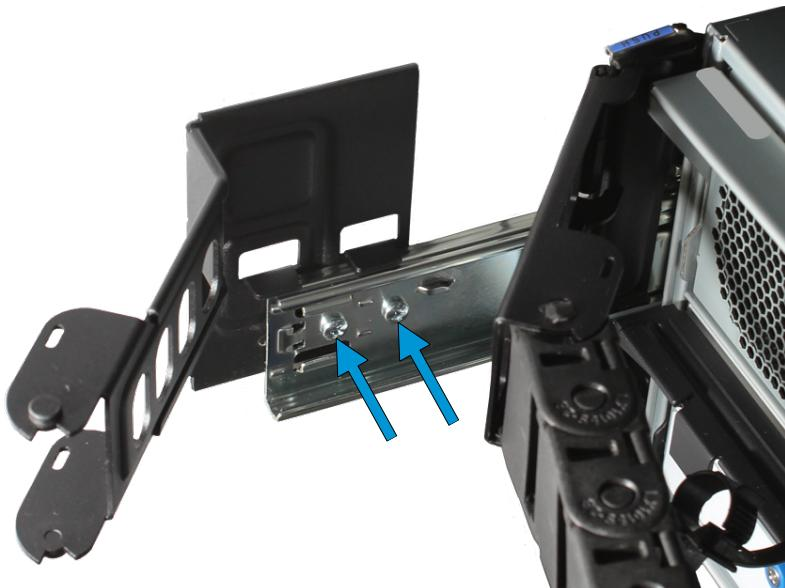
Locate the end of the flex housing with exposed holes. Unclip and open the two tabs closest to the end so the flex housing can expand enough to fit over the bracket pins. Press the flex housing firmly into the bracket until the holes seat on the pins.
