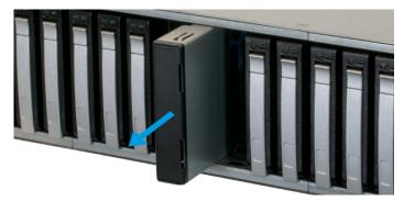
Each drive tray has two indicator lights for status and fault. The status light is blue when the drive is active or a hot spare. The fault light is solid red when the drive has an error or an active identify command.
