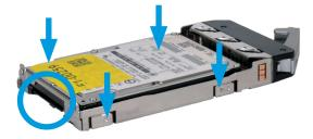
If you purchased fewer than 24 drives with the system, the system has air baffles installed in all remaining drive tray slots. To install new drive trays in the system, remove a baffle by inserting a flathead screwdriver in the baffle grooves, then gently push the baffle out. For proper airflow, we recommend you keep all baffles in place unless you are installing new drives.
