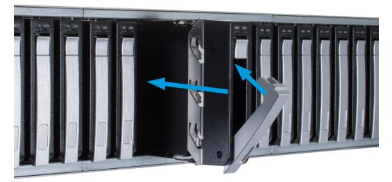
To remove a drive tray, press the button to open the latch, then gently swing the latch open and pull the tray out.
