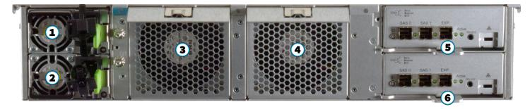
From left to right, the back panel has two power supplies, PSU1 (1) and PSU2 (2), case fans FAN1 (3) and FAN2 (4), and expansion controller 1 (5) and 2 (6). Expansion controllers have several ports and indicators:
