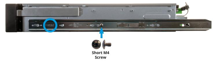
Follow this procedure to slide out and attach the second chassis rail to the other side of the system.
