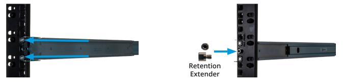
With the front of the rail installed, extend the back of the rack rail towards the equivalent attach points on the rear rack post. Make sure the rail remains level from front to back. Follow this process to install the other rack rail.
