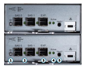
Each expansion controller has an ID button (1), two HD Mini SAS3 connectors for connection to a host (2), another HD Mini SAS3 connector for expansion (3, not used), controller status light (4), and a mini jack for an RS-232 serial connection (5).
