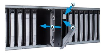
To remove a drive tray, press the button to open the latch, gently swing the latch fully open, and slide the tray out of the system.
