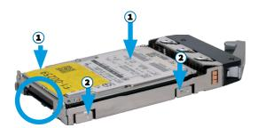
To insert a drive in a tray, align the drive connectors with the rear of the tray and drive side screw holes with the trays retention pegs. Push the drive side screw holes into the fixed retention pegs (1) then into the flexible retention pegs (2). The drive will click into place.
