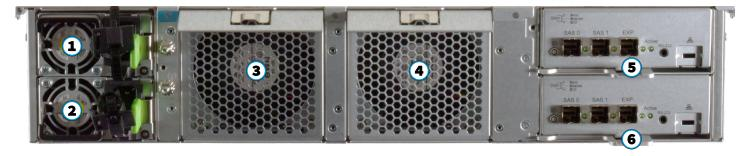
From left to right, the back panel has two power supplies, PSU1 (1) and PSU2 (2), case fans FAN1 (3) and FAN2 (4), and expansion controller 1 (5) and 2 (6). Expansion controllers have several ports and indicators:
