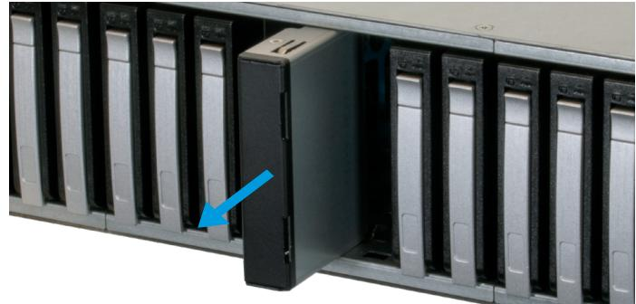
Each drive tray has two indicator lights for status and fault. The status light is blue when the drive is active or a hot spare. The fault light is solid red when the drive has an error or an active identify command.
