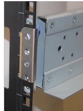
**Caution: Two people are required to safely lift the chassis for rack installation or removal.** Do not install drives until after the chassis has been installed in the rack, and remove all drives before removing the chassis from the rack. Carefully place the chassis onto the rails mounted in the rack. Push the chassis in until the ears are flush with the front of the rack. If needed, attach the bezel. Use two of the supplied screws to secure each ear to the rack.
