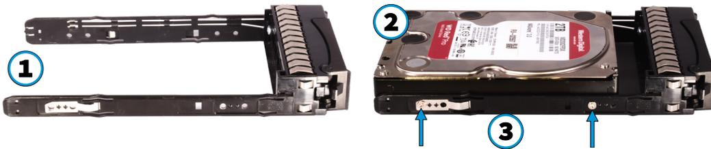
Place the tray on a flat surface (1), mount the hard drive into the tray with the connector to the rear of the tray (2), and secure the hard drive in the tray with four screws, two on each side. (3).
