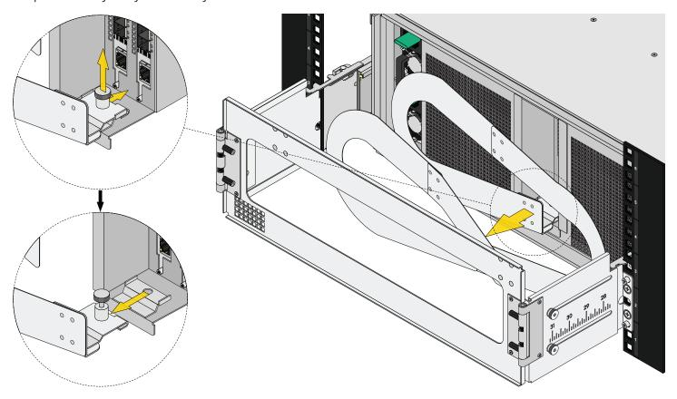
Pinch the spring pegs on the CMA hinge together and pull it away from the bracket. Repeat for the other side.
