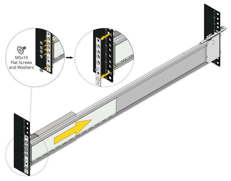
At the rear, remove both M5 X 10 flat screws with washers, then swing the blue latch handle open and extend the rail away from the rack post. Repeat this process for the other rail.
